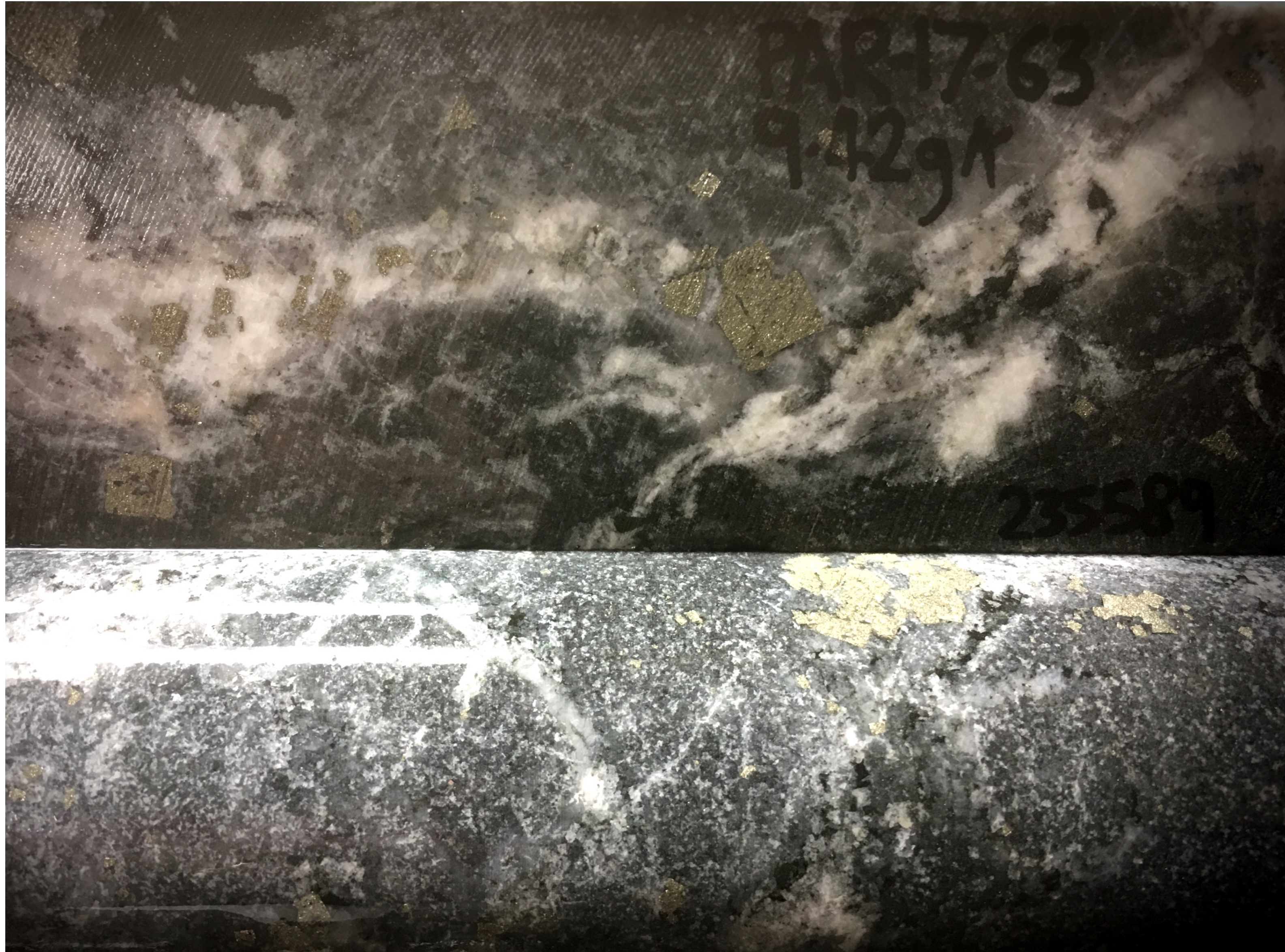
"High Grade" Magnetic Diorite Core Example with Clotty Pyrite
