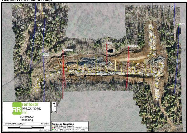
The channel sampling, carried out after stripping overburden which varied between 0 and 3m in depth, has revealed consistent nickel/cobalt mineralization, similar to what has been seen in the near surface drilling to date, however, it has also resulted in a greater proportion of copper/zinc intersections than seen in drilling. Exploration continues on this >5km polymetallic system, located within a 20km magnetic anomaly, where Renforth has only drilled 5,626m.
